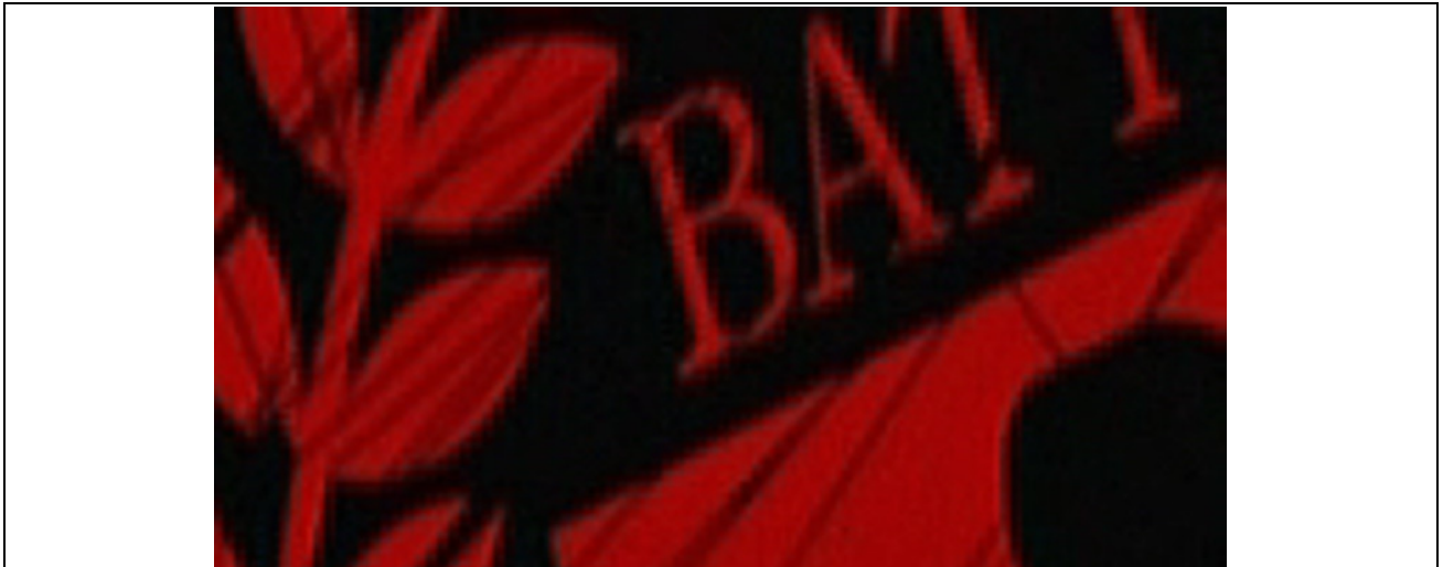
figure 2a: example of progressive source (YV12) being upsampled as interlaced video (YUY2)
